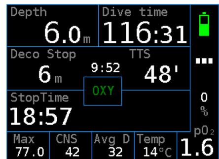
Setting of fresh/sea water doesn't affect decompression calculations. Decompression is based on ambient pressure and is independent of displayed depth. Only depth of decompression stops is rounded up to usual values according to settings of fresh/sea water and metric/imperial units.
