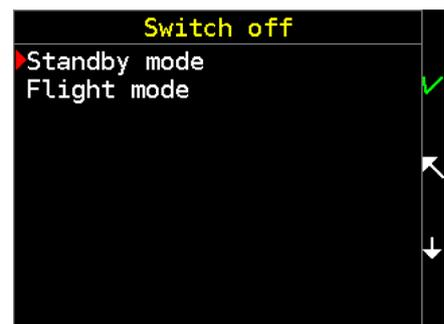
Upon surfacing the Freedom will switch to surface mode after time set in the dive termination timeout. Then it will switch to standby mode after time set in the surface idle timeout. Pushing any button restarts the idle timer in the surface mode.
