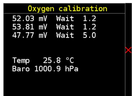
It is preferred to calibrate O<sub>2</sub> sensors prior each dive. Do not use sensor reading from sensors calibrated more than three days ago.
